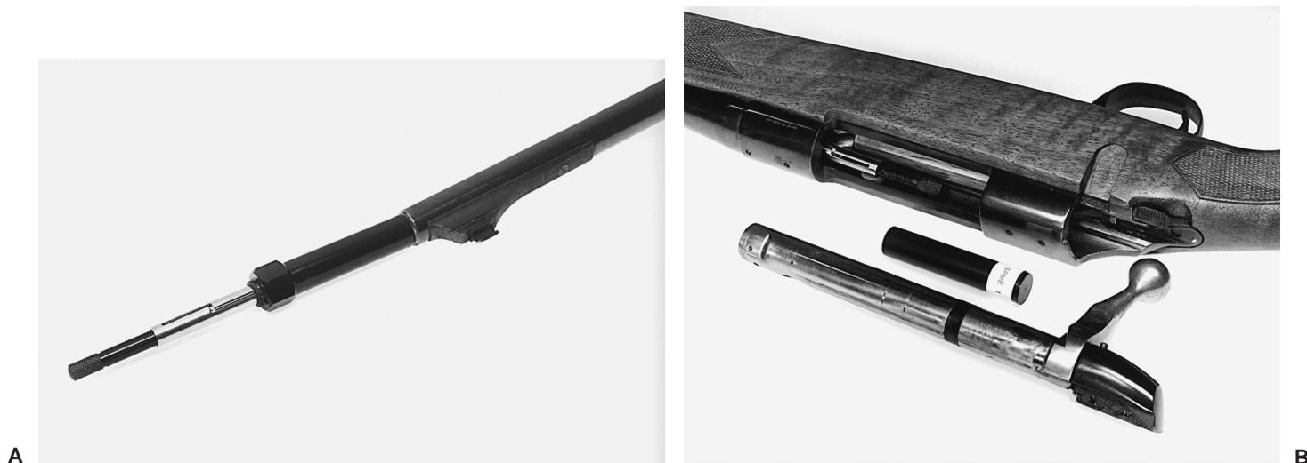
FIG. 1—Sampling from rifle barrels. The SPME fiber is exposed to the atmosphere inside the barrel for 20 min at room temperature. The rifle shown is of .30–06 caliber: (a) sampling at the muzzle position; (b) sampling at the breech position. Note that the bolt of the rifle must be removed as well as the adjustable depth gage from the SPME holder. The SPME device is pushed inside the barrel using tweezers.
